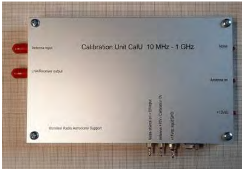
Fig. 7: Calibration unit containing semiconductor switch and a noise source. Unit will be supplied with a calibration table and free Python script to control the unit as well as to calibrate FIT-files from CALLISTO.
