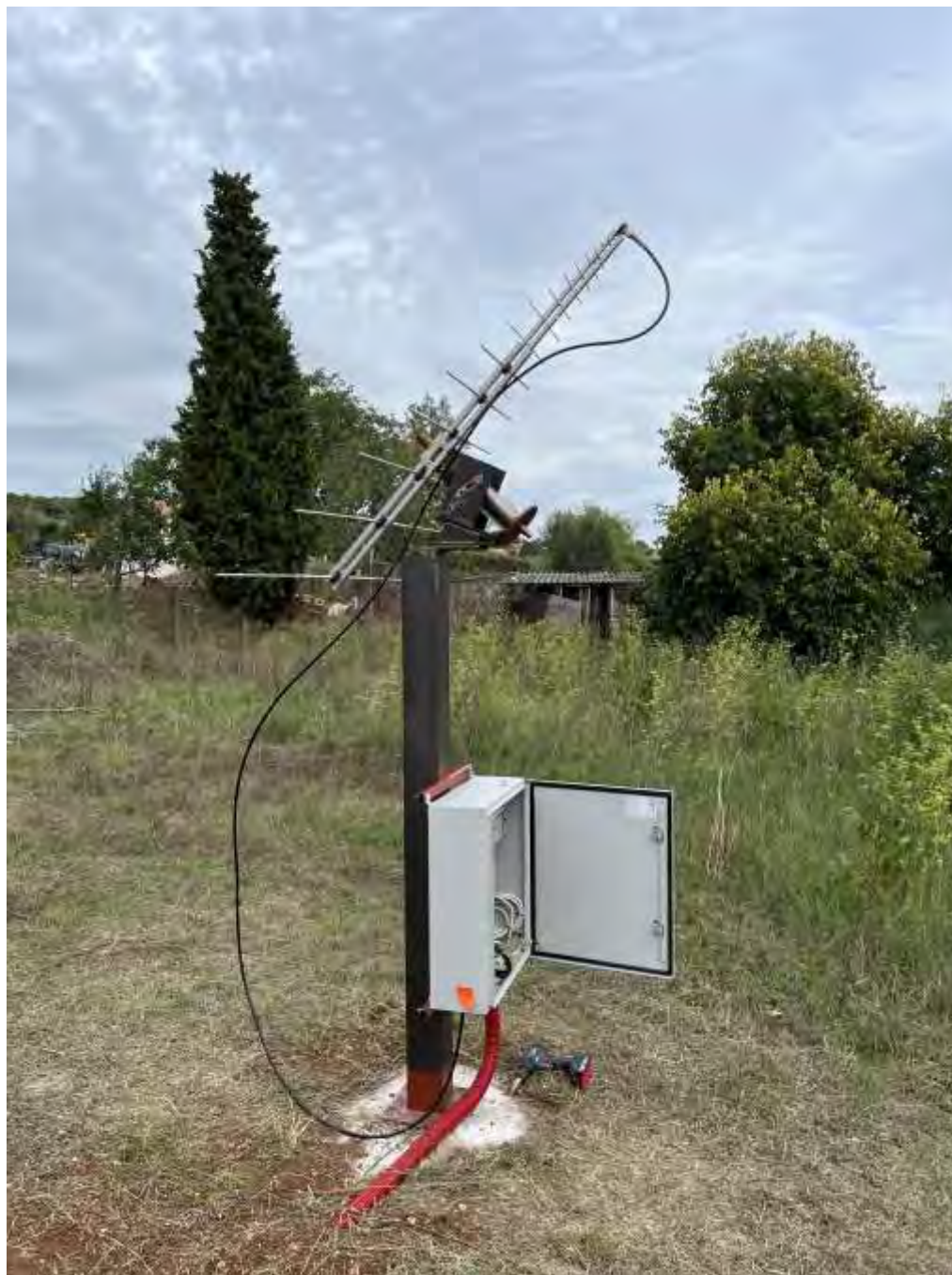
Fig. 5: Logarithmic periodic dipole array (LPDA) including front-end box containing low noise amplifier. Antenna with tracking system. Station: Croatia-Visnjan Contact: Marko Radolović < mradolovic(at)gmail.com >
