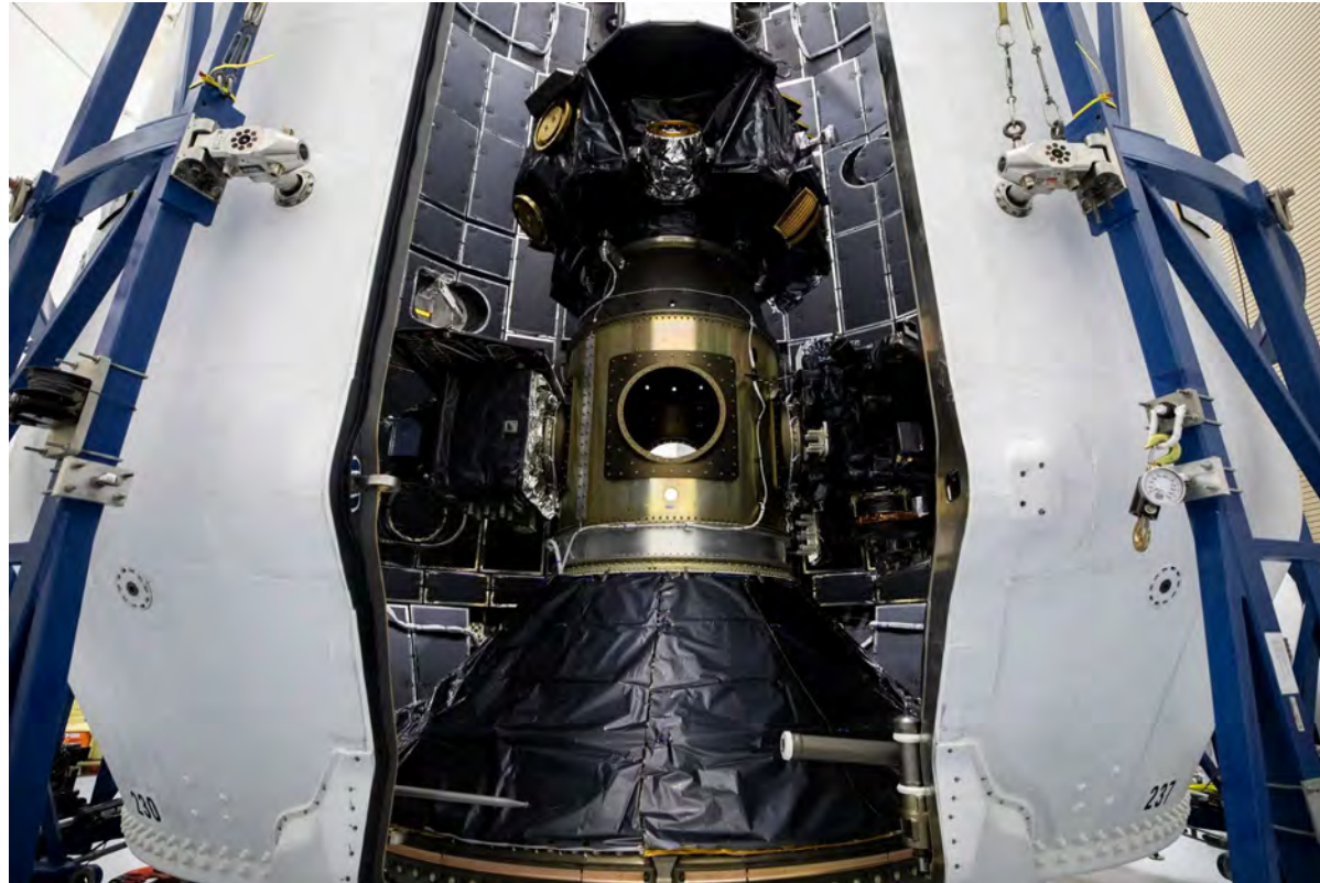
NASA's Interstellar Mapping and Acceleration Probe, along with two spacecraft, during encapsulation inside a SpaceX Falcon 9 rocket at the Kennedy Space Center in
