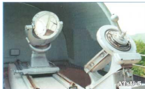
Horizontal solar telescope "ATsU-5"
