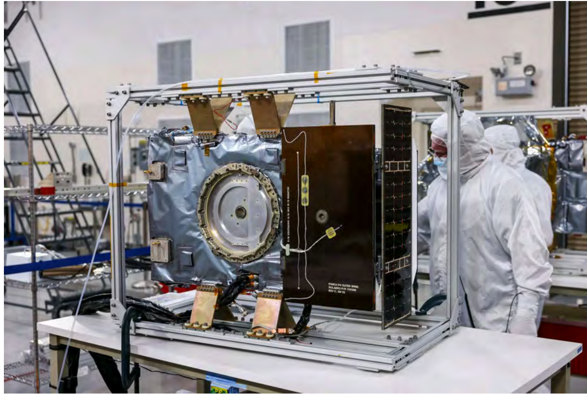
A solar array deployment test on one of the PUNCH satellites at Astrotech Space Operations on Vandenberg Space Force Base in California last month. Alex Valdez/USSF 30th Space Wing/NASA
