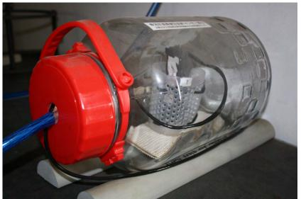
A second fluxgate magnetometer was built at GRL in 1987, improving the first design, the analogue output was between  $\pm$  10 volts equivalent to  $\pm$ 500nT. After recording test made at Kakioka Magnetic Observatory this Magnetometer was installed Huancayo Observatory in March of 1988. Recording on a PC based data acquisition system equipped with a 12 bits ADC and an own software developed for data acquisition. Actually it is working at Ancon Observatory.
