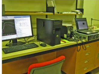
Installation of the data-analysis PC (including IDL and Solar Software) and data-storage system (RAID5)
