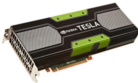
Tesla K20X in 2012 (dp:1.31TFlops, sp:3.95TFlops)
