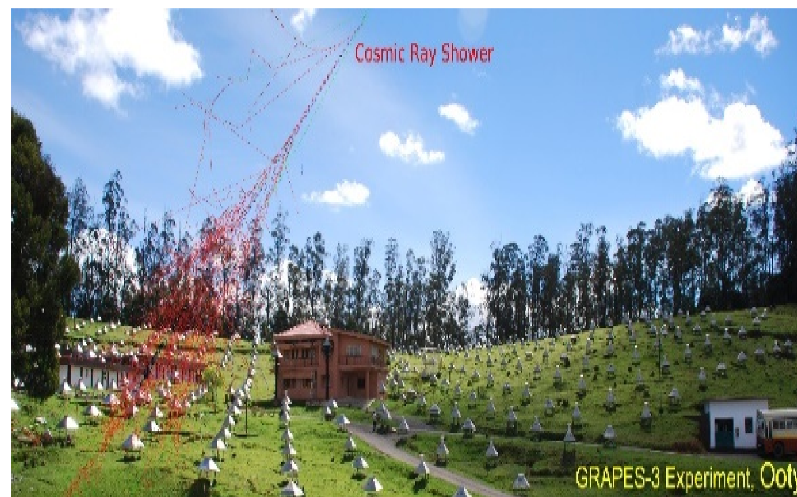
View of the GRAPES-3 experimental site showing scintillator detector array, control room building (center) and muon detector buildings (left)
