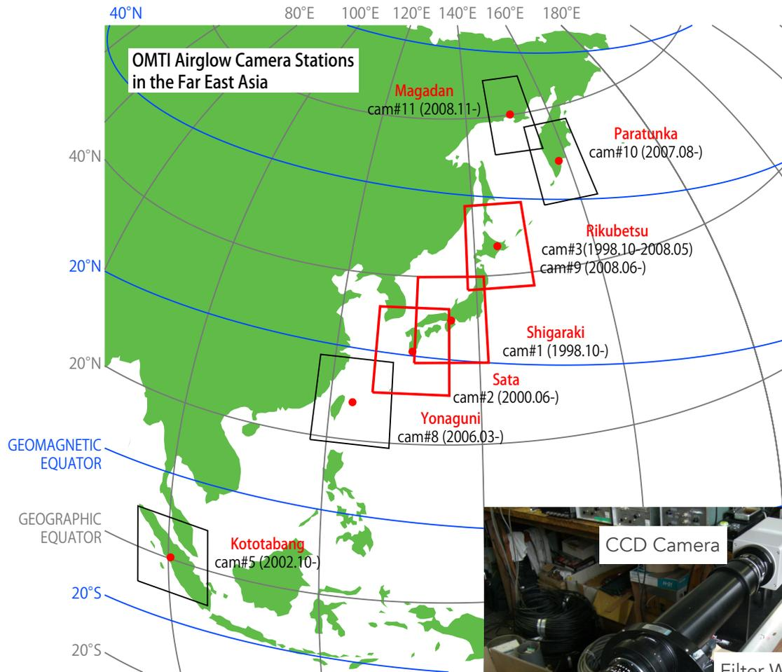
Optical Mesosphere and Thermosphere Imagers (OMTIs) have monitored mesospheric waves and ionospheric structures.
