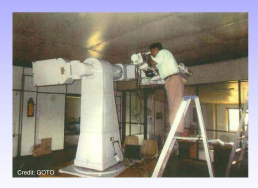
Sri Lanka astronomer adjusting CCD spectrograph for the reflector.
