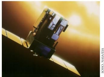
The SOHO spacecraft provides us with an early warning system for detecting disruptive solar activity
