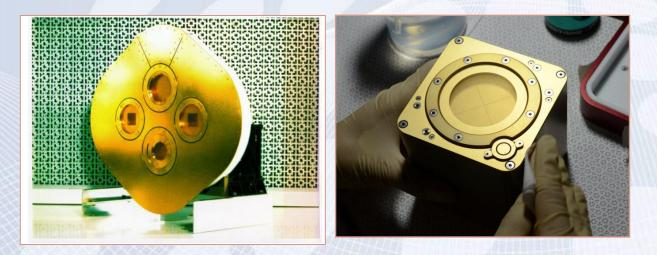
The Ionospheric Electrodynamics and Plasma Instrument (IPEI) on board the Formosat-1 satellite (left) and the allin-one miniature Advanced Ionospheric Probe (AIP) on board the upcoming Formosat-5 mission (right).
