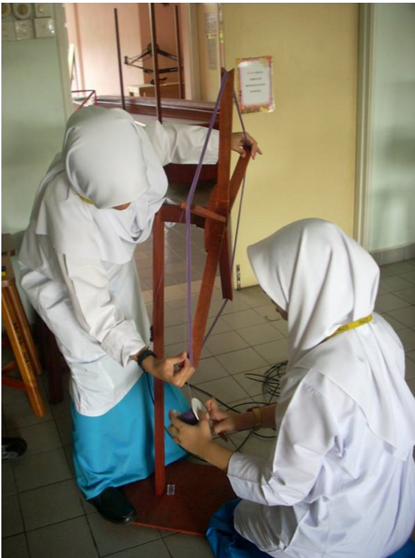
Fig. 1. Students making the VLF loop antenna to capture the VLF signal from various VLF transmitter stations. This loop antenna is 1\text{ m}^2 in diameter, with 29 turns.
