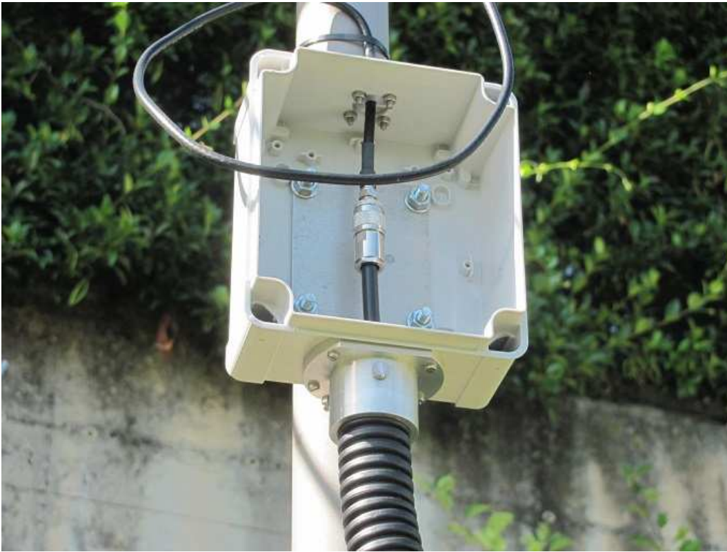
Fig. 4: Example on how to install a frontend between antenna and Callisto. Here in this example at IRSOL in Switzerland antenna is directly connected to Callisto due to high level of local rfi. But there is enough space in the box to install a low noise amplifier in the future. Congratulations for this nice example to: Mari Gianpaolo, collaboratore tecnico, IRSOL , gpmari(at)irsol.ch , Istituto Ricerche Solari, Via Patocchi 57, 6605 Locarno Monti. See also the nice cable flanges at the bottom and a similar one at the top. Many thanks, Gianpaolo!
