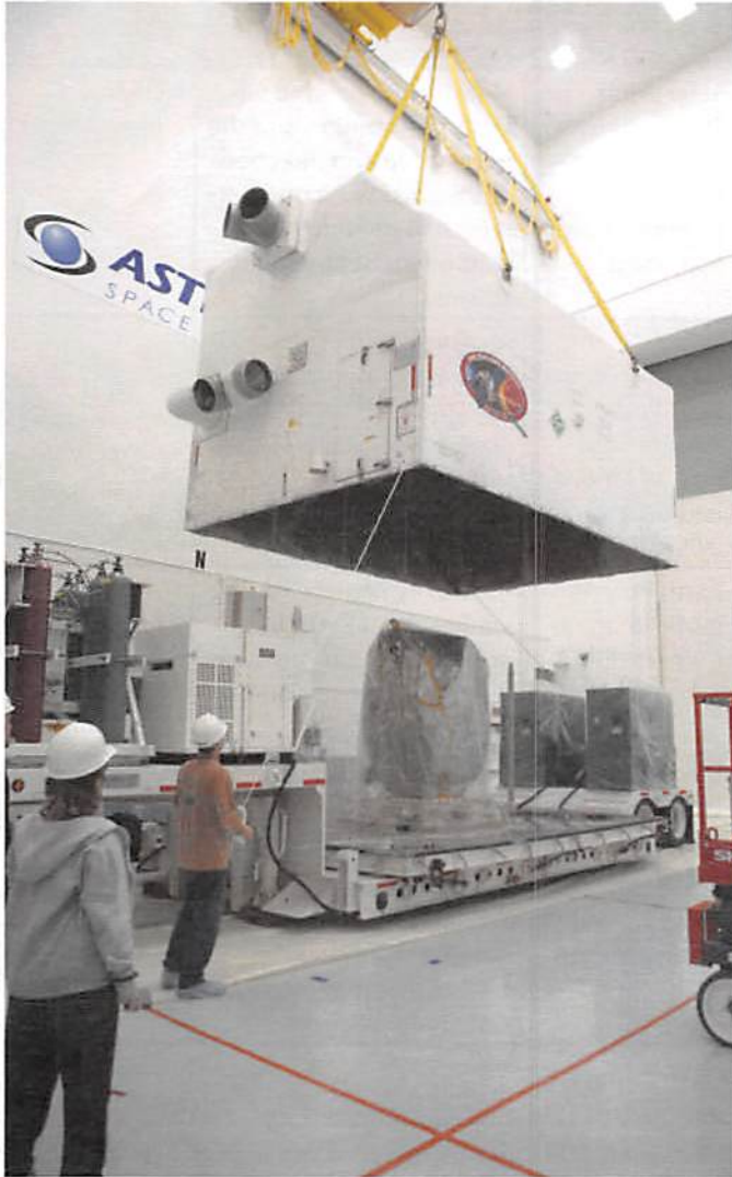
NOAA's Deep Space Climate Observatory spacecraft, or DSCOVR is being unwrapped for the New Year and prepared for launch. In this photo, DSCOVR, wrapped in plastic, comes into view as the protective shipping container is lifted from around the spacecraft at the Astrotech payload processing facility in Titusville, Florida, near NASA's Kennedy Space Center. Photo credit: NASA
