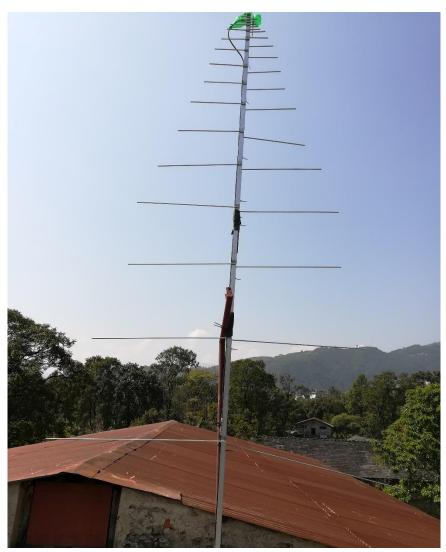
Figure 3: Antenna pointing to zenith, mounted on the top of science building in Pokhara.
