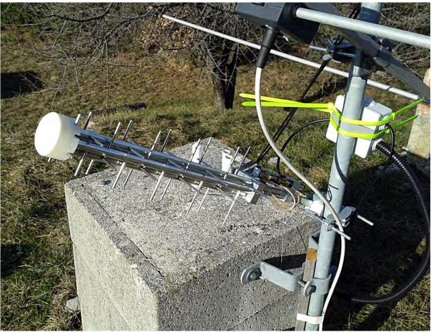
Fig. 8: Detail of L-band antenna 1.0 - 1.6 GHz (LPDA).
