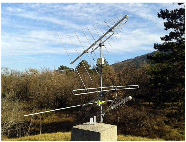
Fig. 7: Antenna farm with new L-band antenna to observe 1.0-1.6 GHz
