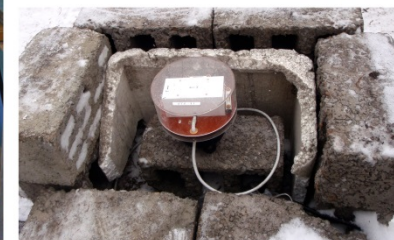
Installation of MAGDAS-9 and DCR-3 magnetometers at ZYK in October 2013.
