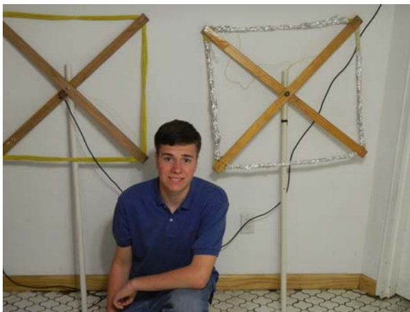
Figure 1. Antennas built to obtain Very Low Frequency waves
