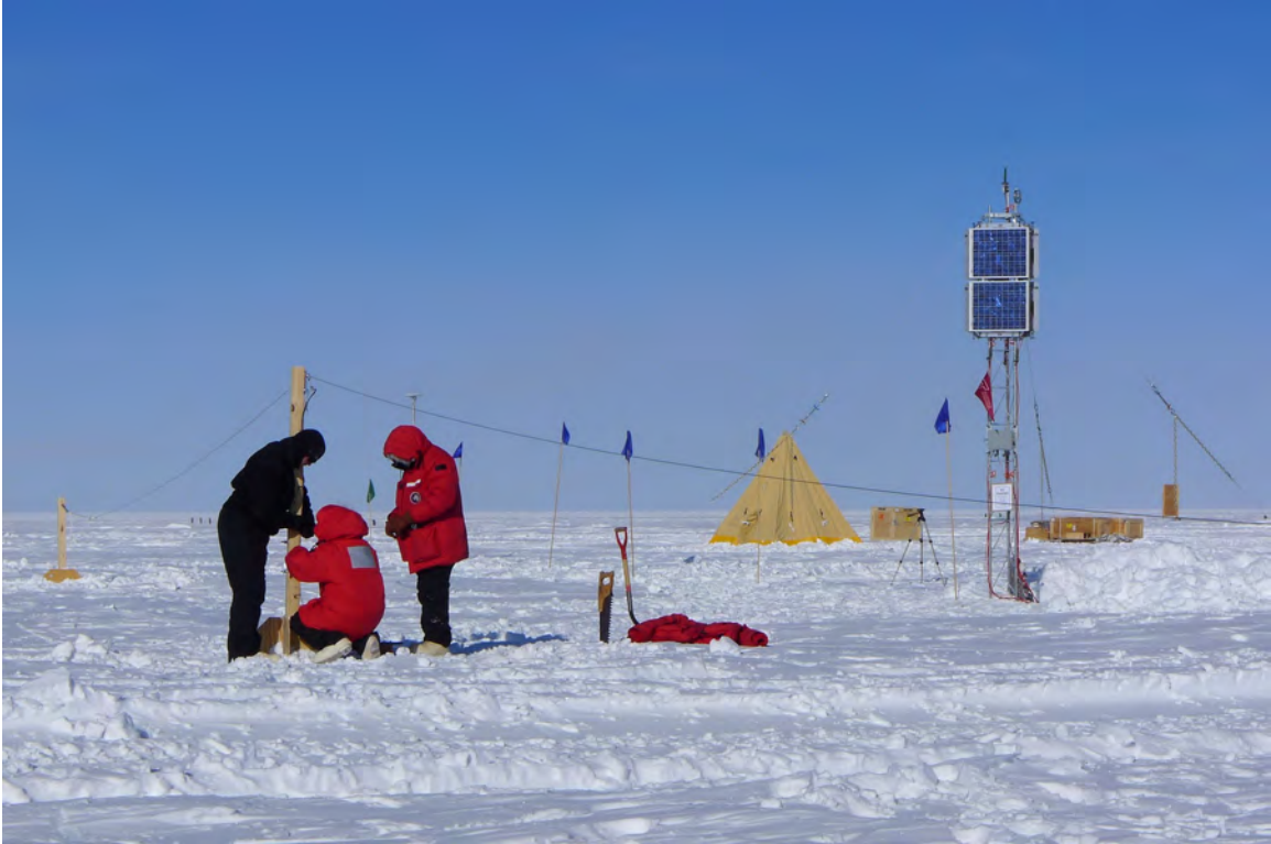
Figure 12. HF dipole antenna installed near the AAL-PIP tower.
