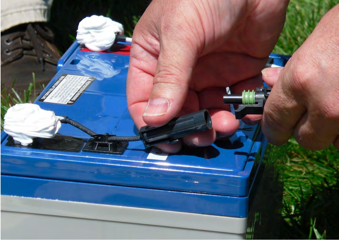
Figure 16. Quick-snap connectors used for battery harness.
