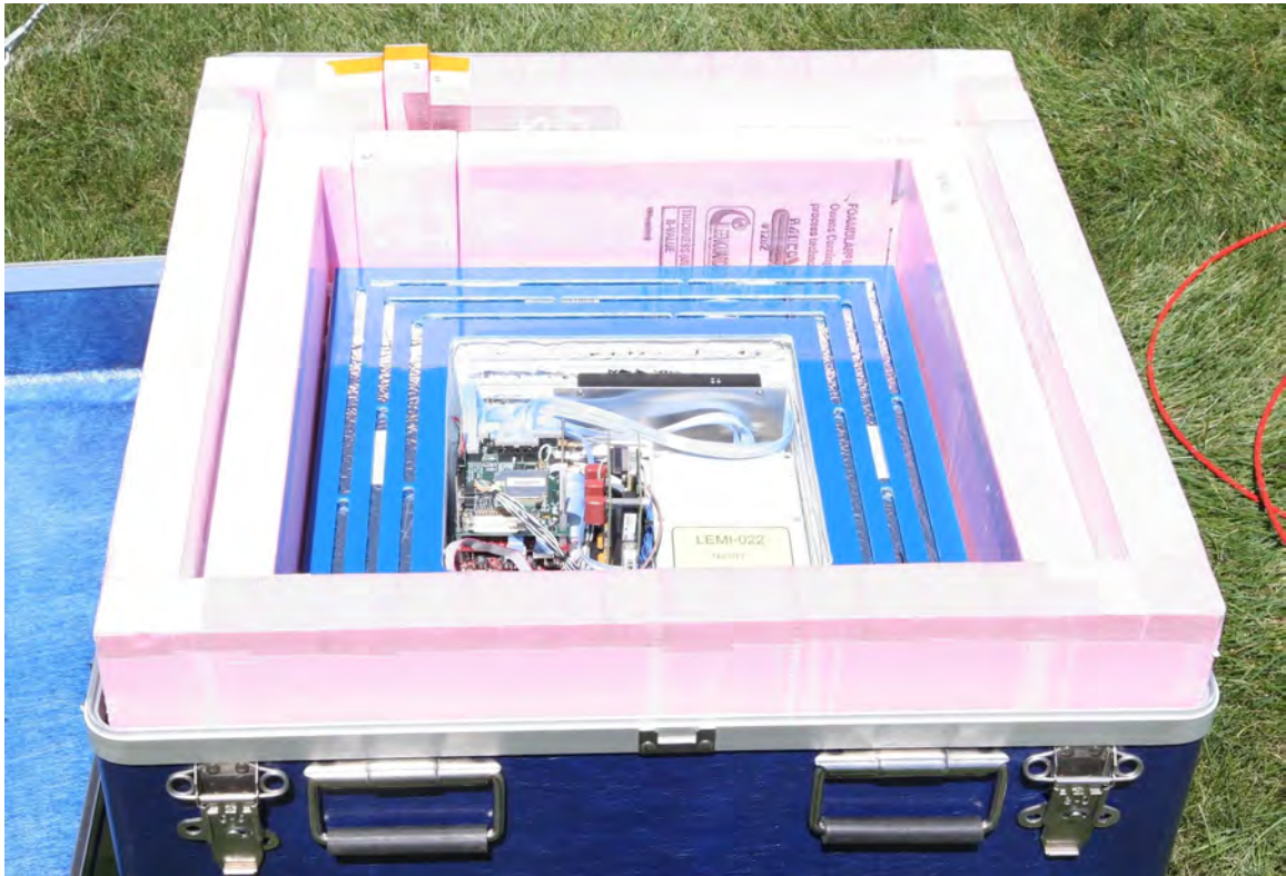
Figure 5. AAL-PIP electronic box containing the single board computer, GPS receiver, HF receiver, magnetometer circuits, and Iridium modem. The electronics is insulated by the vacuum panels.
