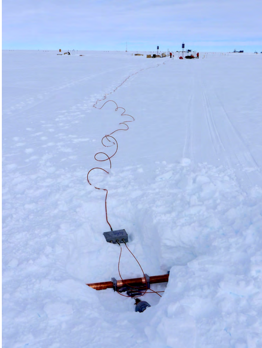
Figure 10. AAL-PIP search-coil magnetic sensor located in a snow pit. The main structure of the AAL-PIP system is in the background.
