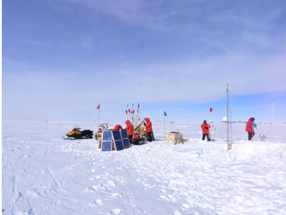
Figure 33. Taking down the AAL-PIP system (Sys6) at the South Pole for the preparation of remote field installation.
