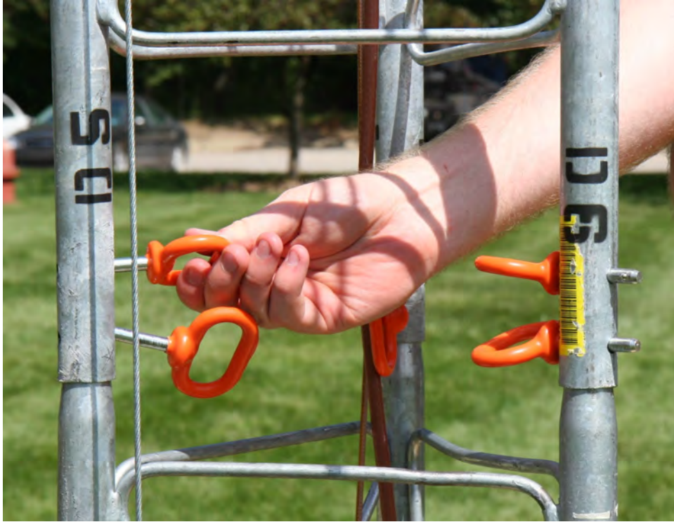
Figure 13. Pins used for tower assembly.
