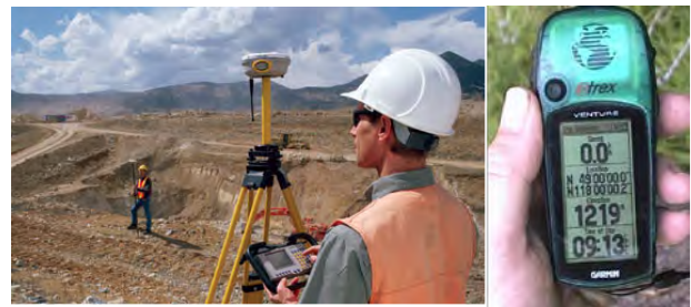
Figure 5-3. GPS precision surveying. (Source: http://www.gps.gov )
