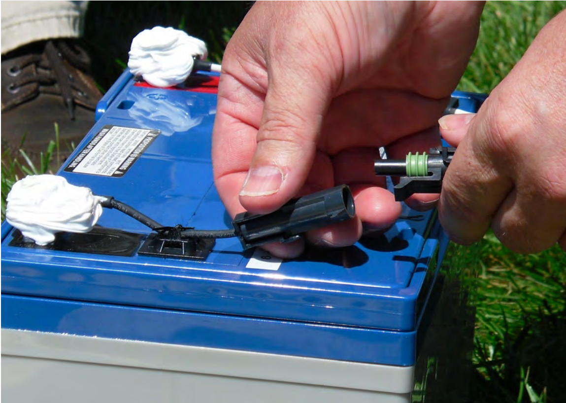
Figure 16. Quick-snap connectors used for battery harness.
