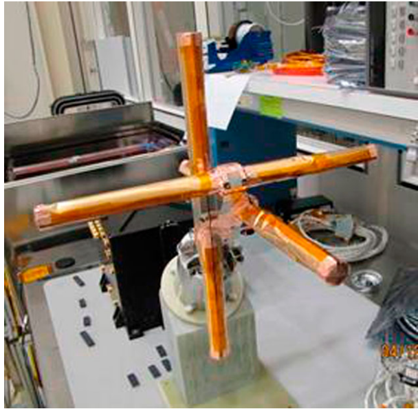
Fig. 14 The Magnetic Search Coil (MSC) sensor assembly and preamplifiers
