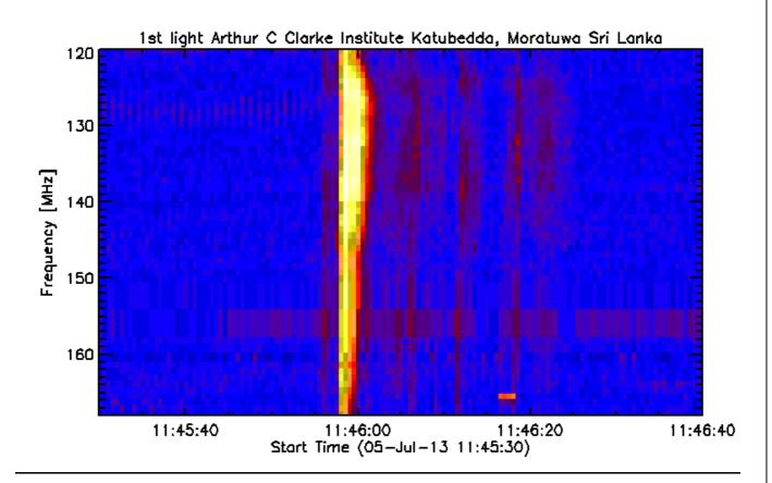
Fig. 6: 1st light of Callisto in Sri Lanka, a type III burst. X.axis time stamp denotes to Sri Lanka local time. In the mean time the system is correctly working in UT.
