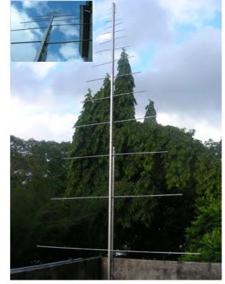
Fig. 4 Log – Periodic a Antenna
