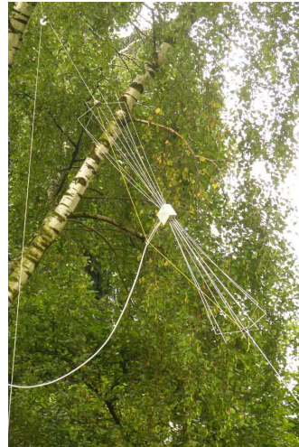
The biconical antenna (called “Fliegenfischfänger” in German language, because it looks like a trap for flying fishes) mounted to a tree. The antennas directional sensitivity should follow the sun, so no tracking system is needed. (Still waiting for some NEC simulations.
