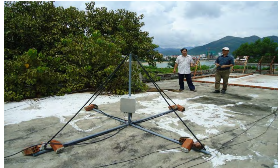
Mounting the Preamplifier Box to the VLF Antenna
