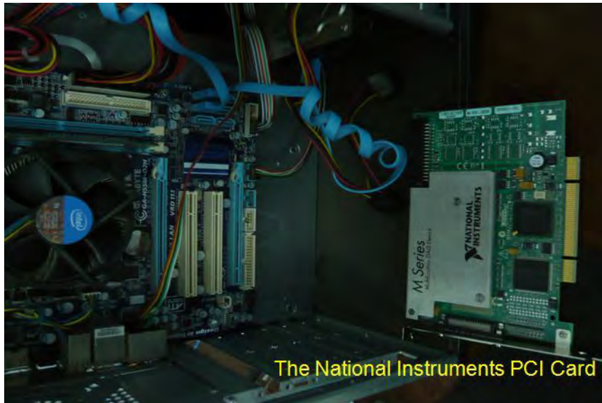
Plug in the card into the PC Main board
