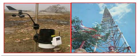
Davis instrument for Atmospheric data collection. Provision of mast for installation of instruments at varying heights.
