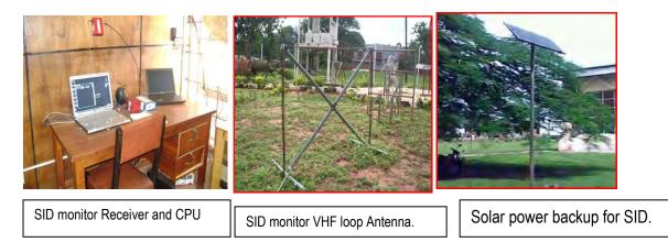
While carrying out lonospheric research, CBSS designed and fabricated a cheap and effective SID monitor.
