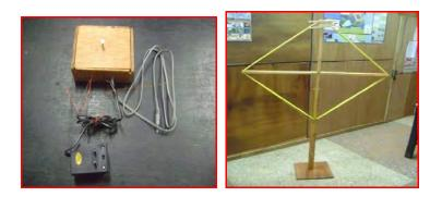
Cheap and effective SID monitor fabricated by CBSS Engineers
