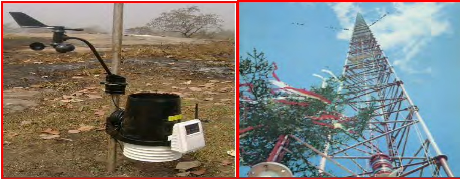
Davis instrument for Atmospheric data collection. Provision of mast for installation of instruments at varying heights.
