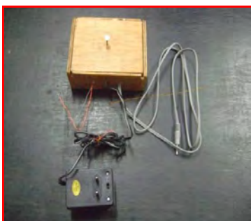
Cheap and effective SID monitor fabricated by CBSS Engineers
