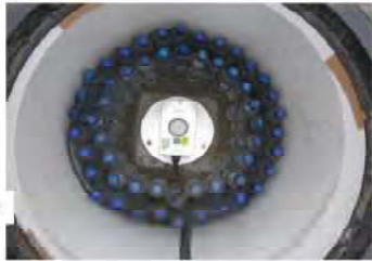
Figure 8: Preparation of water bottles inside sensor casing to minimize temperature drift effects and function as a coolant
