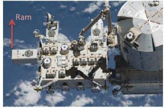
Fig. 5. The Japanese Experiment module has both ram and wake facing attachment points for exposed facilities (courtesy JAXA<sup>8</sup>).
