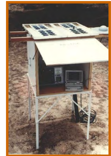
Magnetotelluric station H,D,Z, Ex,Ey components
