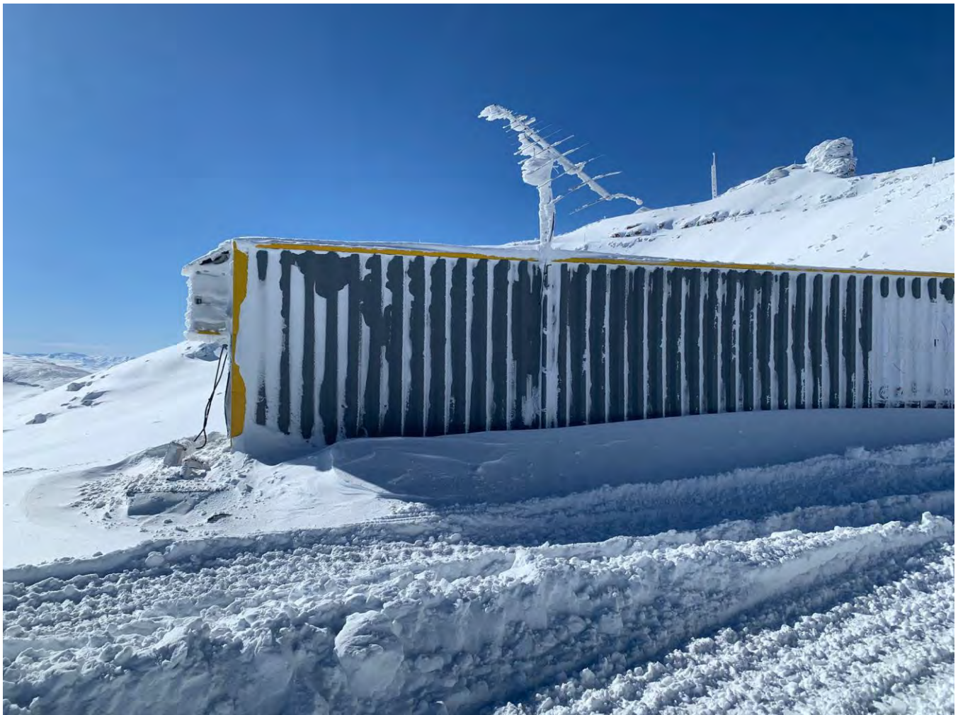
Fig. 1: Logarithmic periodic dipole array (LPDA), suffering from winter-weather conditions. The current location of the antenna is on a mountain at an altitude of 3100 meters in Erzurum, far from the city center in turkey. Image: Dr. Onur Satir
